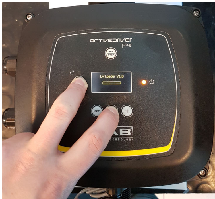
Figure 9B – Updating Active Driver Plus Sw 1.X
